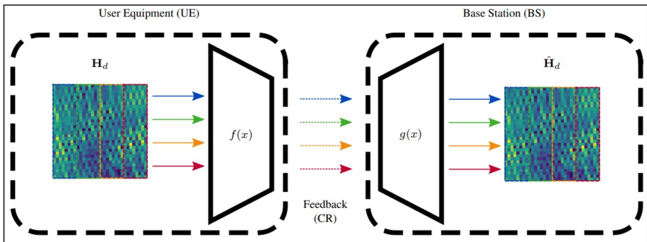
Fig 1: Compressive CSI estimation with model re-use
