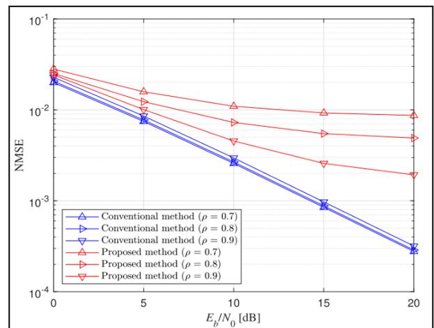
**Fig 4:** Comparison of NMSE performances according to the correlation coefficient,  $\rho$  (nt=64, nr=2 and r=0.969).
