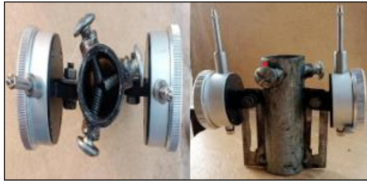
Fig 2a: Picture of slip measuring Device
