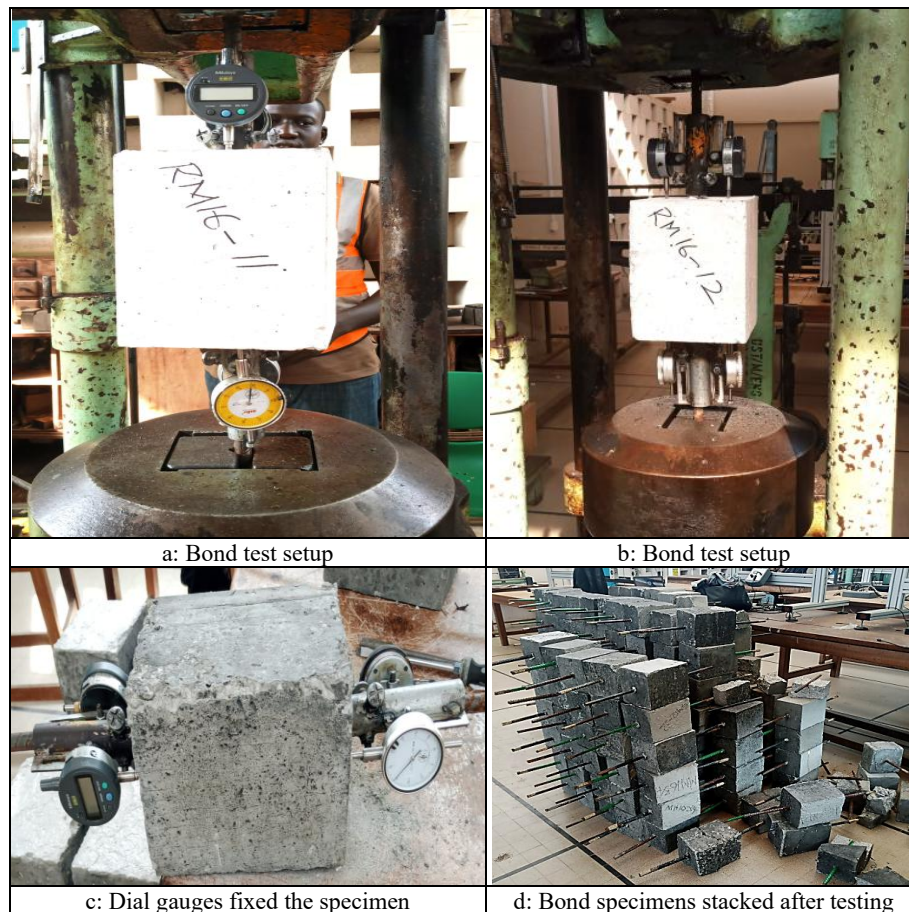
Fig 5: Bond specimen testing setup.
