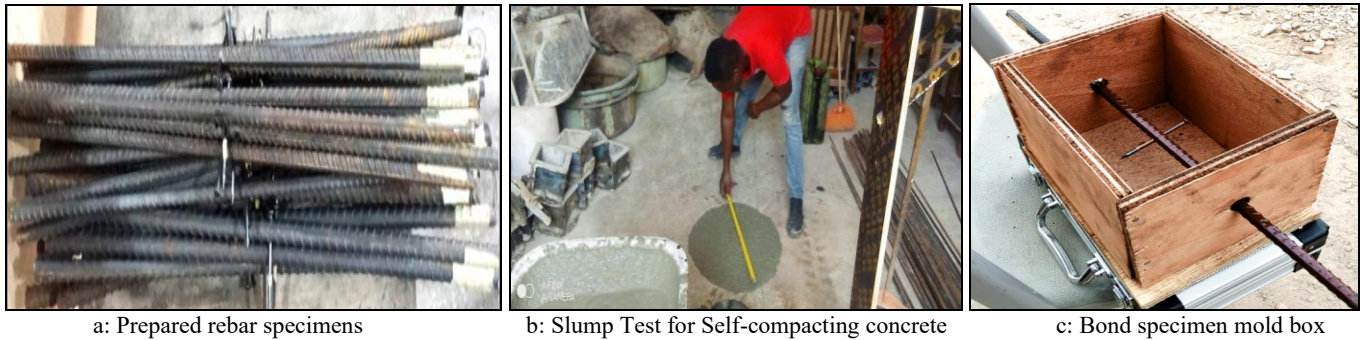
Fig 4: Rebar preparation, coating and geometry information processes.
