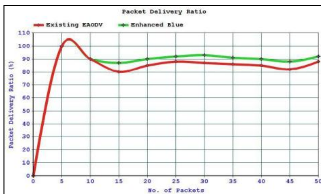
Fig 3: Packet Delivery Ratio comparison between Existing EAODV with enhanced Blue
