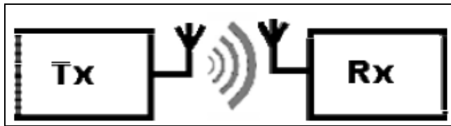
Fig 3: SISO - Single Input Single Output
