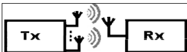
Fig 5: MISO - Multiple Input Single Output
