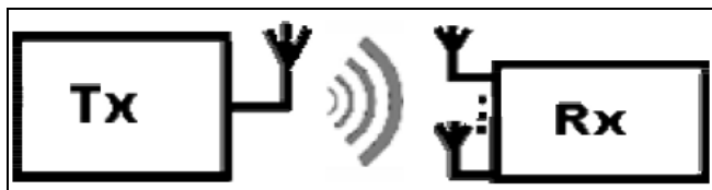
Fig 4: SIMO - Single Input Multiple Output
