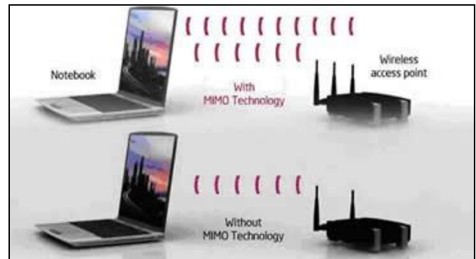
Fig 2: MIMO technology allows for the simultaneous transmission of more data by using multiple radios.
